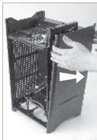
④ Remove the Front Panel by just pulling away from the Case.
